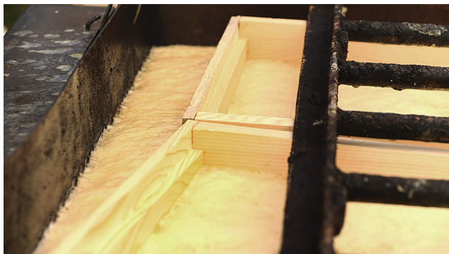
Note the foam caused by the new boxes. We try to leave at least 12” between the top of the wax and the top of the tank, but that is sometimes not enough if the wood is wet or you pack it full with lots of small pieces. Photo by Kirk Mason
